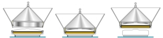
1. Before Capping 2. Cone leveled and Capped 3. IBC removed
